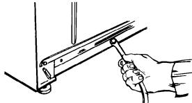
Pull firmly to remove the other "' end of shipping strap from the back of the washer. The shipping strap plug must be completely removed from the washer for the self-leveling legs to be released.
